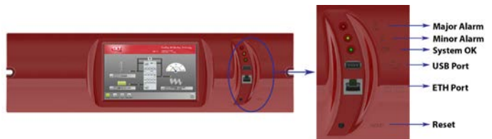
Figure 5. CATENA - Front Details
